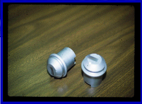
Glass forming tools. This nodular deposit performs well in applications requiring release & abrasion resistance.
