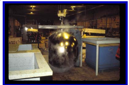
36" diameter ball valves. TM 103 provides a uniform corrosion resistant coating for the petroleum industry.
