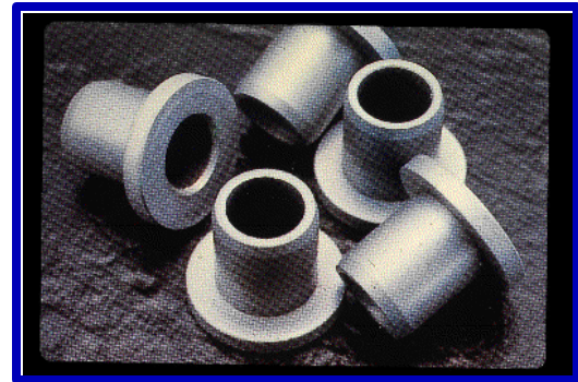
The nodular chrome deposit retains oil like cast-iron from high wear areas.
