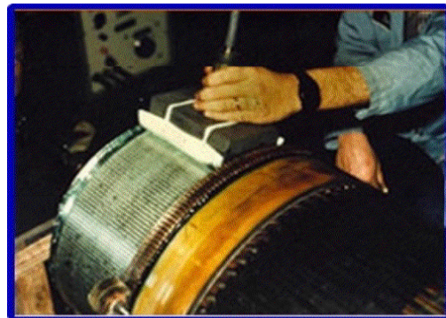
Worn armature plated to size on site.
