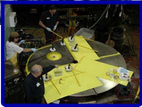
9,000 pound mold selectively brush plated on site for corrosion resistance.
