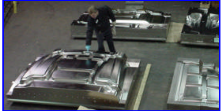
Large Aluminum Molds coated with E-Krome that allow Aluminum to be used instead of Steel or Stainless
