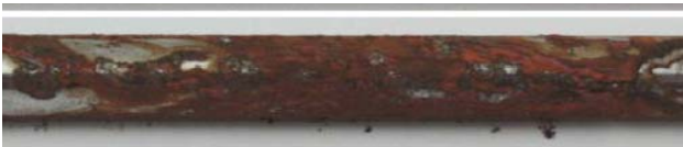
Hard Chrome Corrosion 48 hours results above picture Hard Chrome .0005 inches Thick ( 48 hours)
