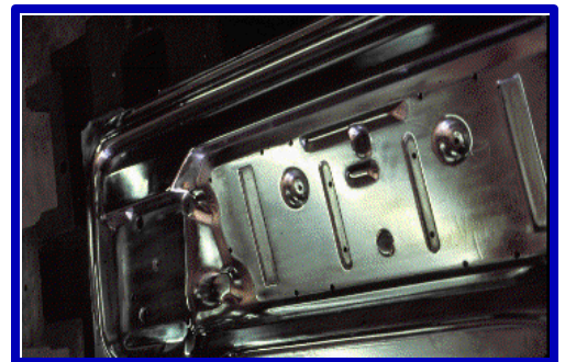
Used on large dies for added wear & anti-galling properties.
